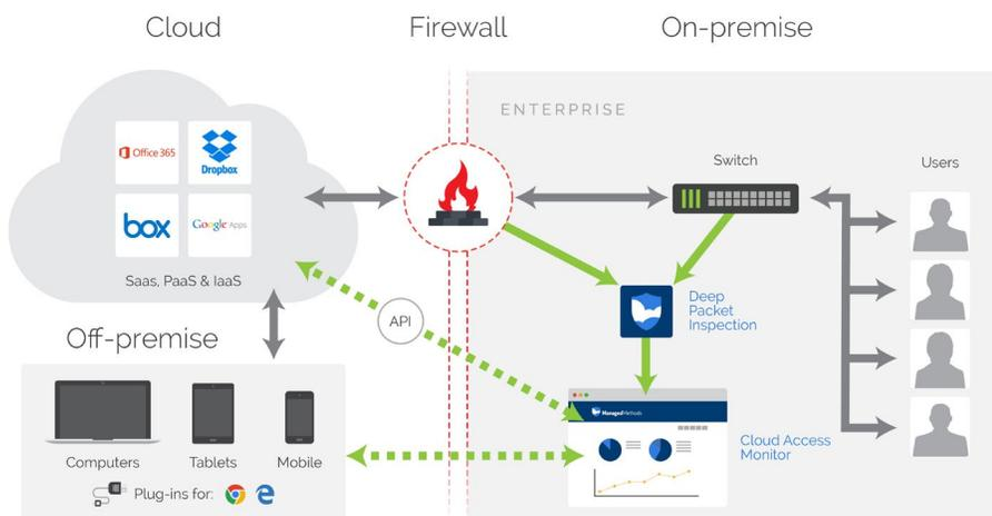
*Figure 1: The Architecture of Cloud Access Monitor*
